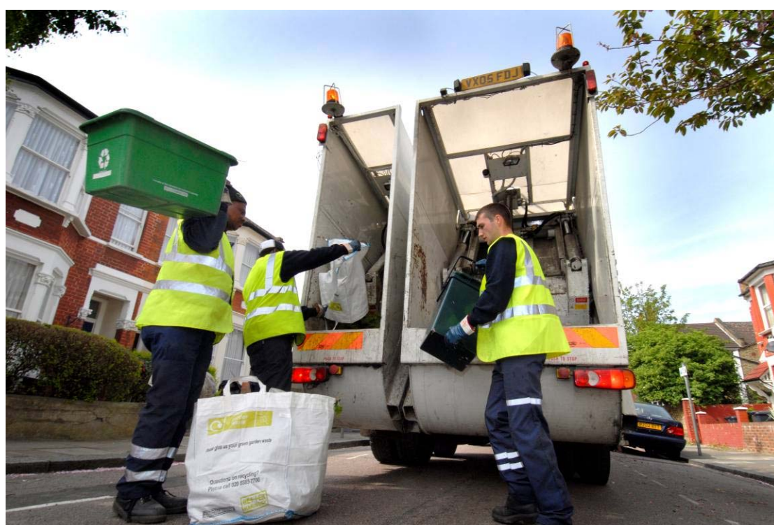
Waste is collected for composting and recycling in some areas using a “split- body” vehicle.
