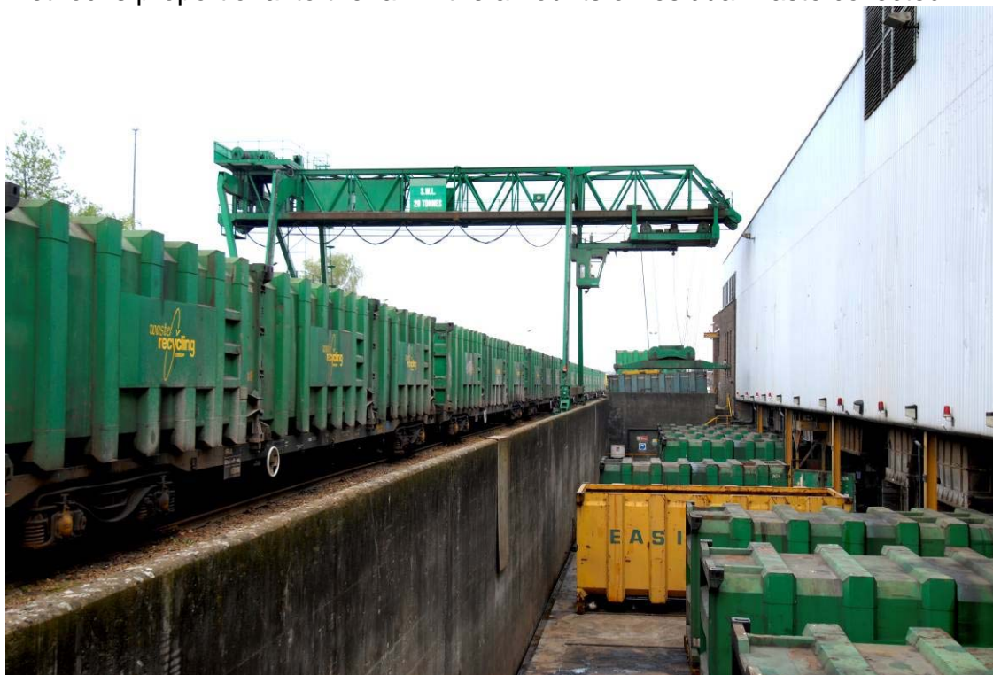
Residual waste is loaded into containers at the Hendon Rail Transfer Station for transfer to landfill.
