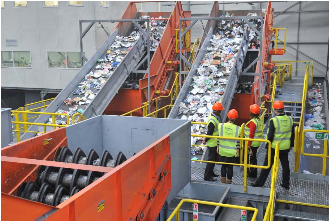
Dry mixed recyclable waste is sorted at a materials recycling facility (MRF).
