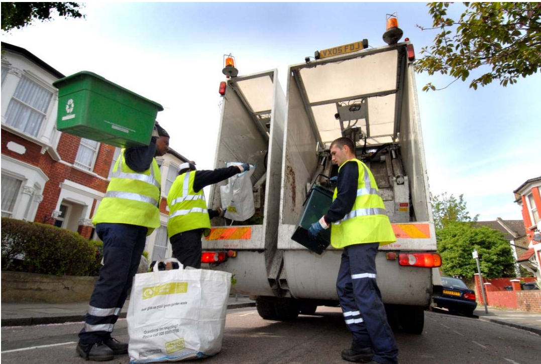
Waste is collected for composting and recycling in some areas using a “split-body” refuse collection vehicle.
