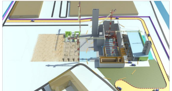
An extract from Acciona's 4D construction sequencing model. Construction is being planned using 4D modelling to optimise sequencing and interfaces with the operational aspects of the EcoPark
