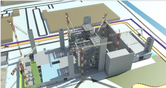
An extract from Acciona's 4D construction sequencing model. Construction is being planned using 4D modelling to optimise sequencing and interfaces with the operational aspects of the EcoPark
