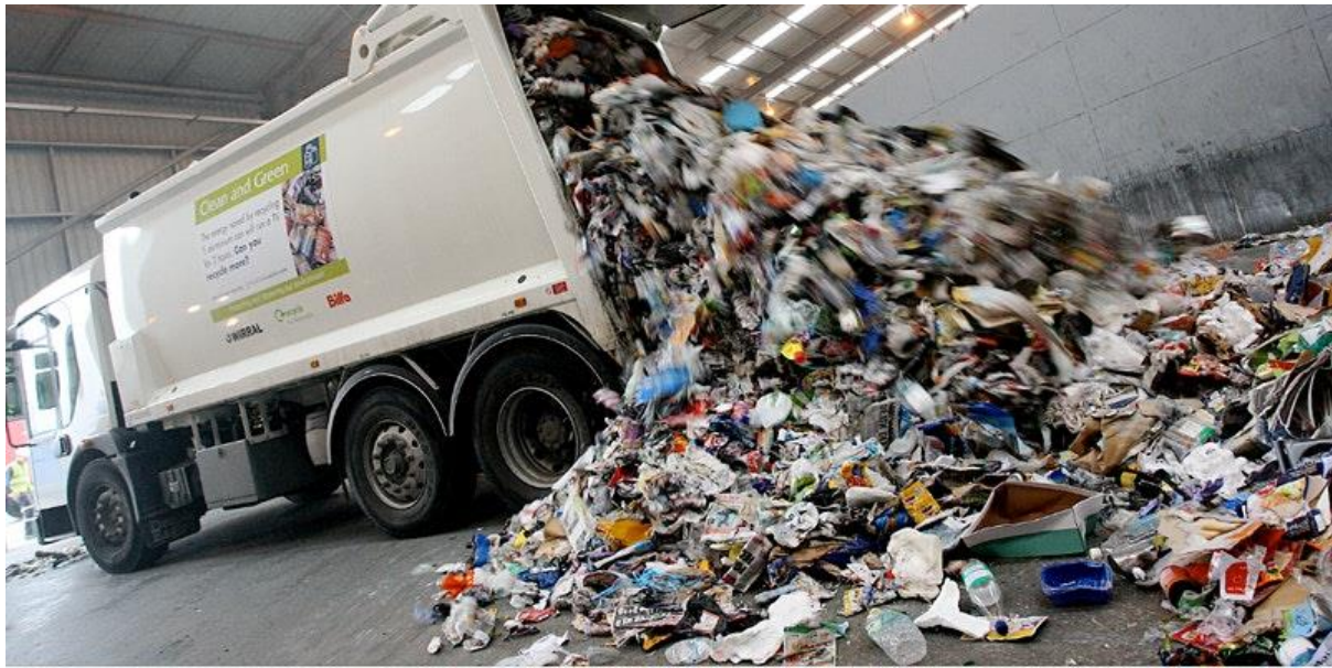
A lorry offloading dry, mixed recycling (DMR)
